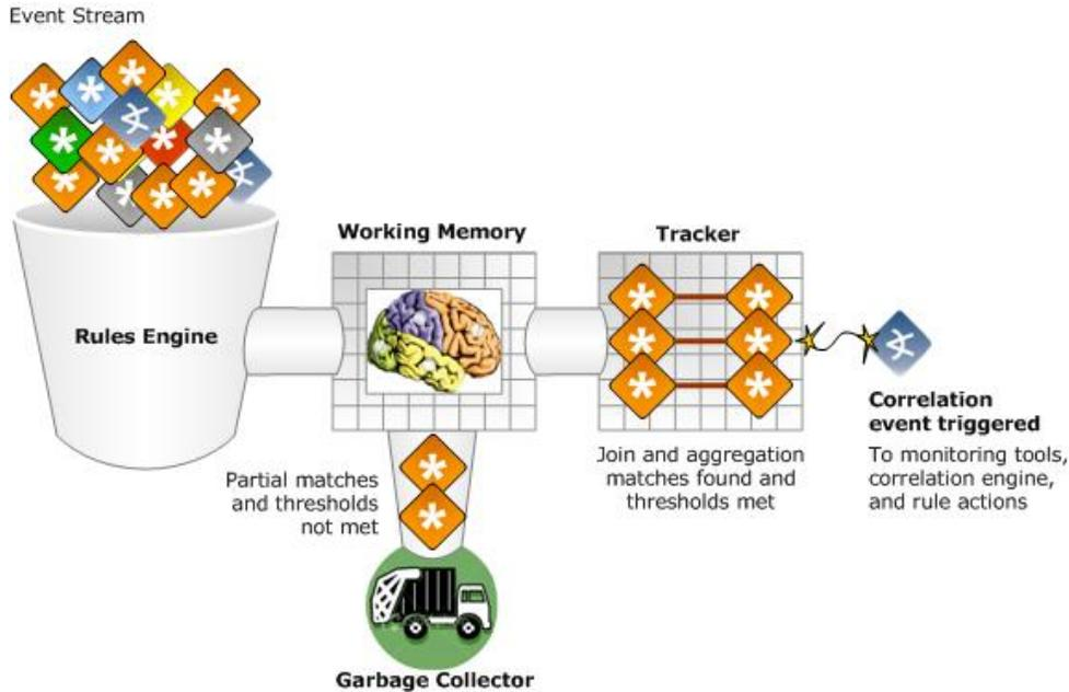
The rules engine evaluates the event stream, holds matches in working memory, and processes join and aggregation conditions in the tracker. If all conditions are met within the time thresholds, a correlation event is triggered.
