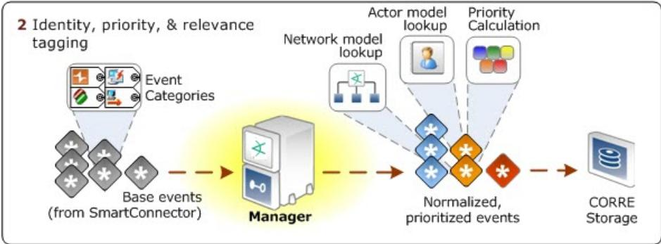
The SmartConnector sends the aggregated and filtered events to the Manager, where they are evaluated and tagged with network and actor modeling information, and priority levels, then stored in CORR-Engine storage.
