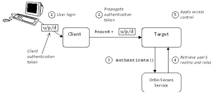
Figure 17: Two-Tier CORBA System in the iSF
