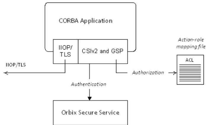
**Figure 16:** A Secure CORBA Application within the iSF
