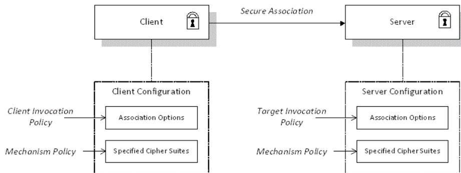
Figure 52: Configuration of a Secure Association
