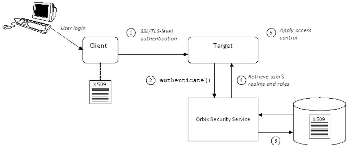
Figure 19: Overview of iSF Certificate-Based Authentication
