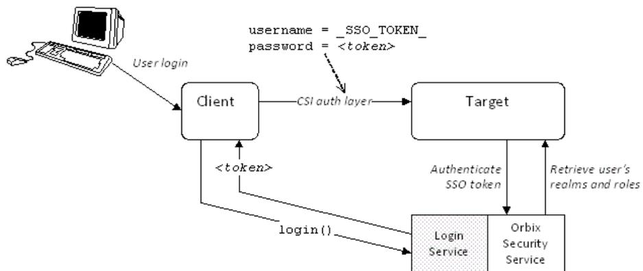
Figure 25: Overview of Certificate-Based Authentication with SSO
