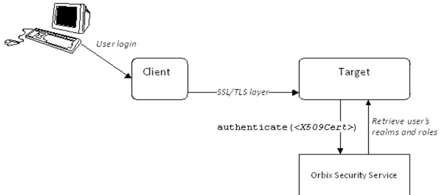
Figure 24: Overview of Certificate-Based Authentication without SSO
