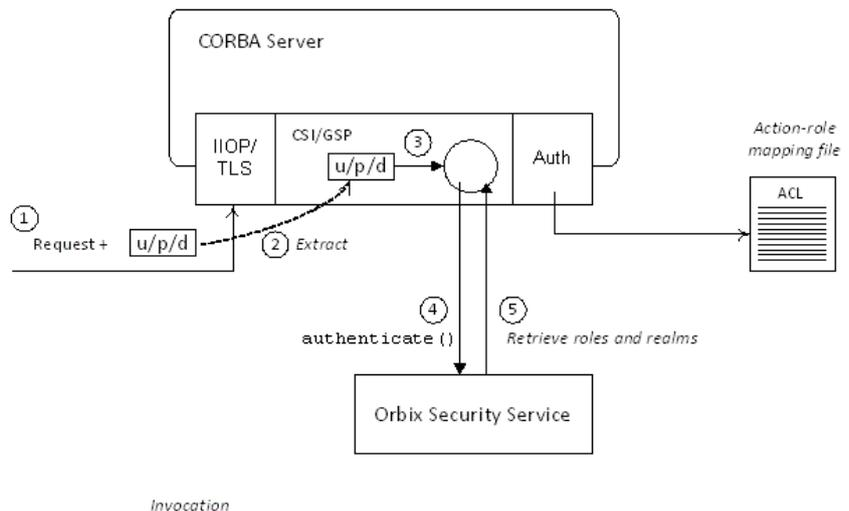
**Figure 65:** CSIv2 in the Orbix Security Framework
