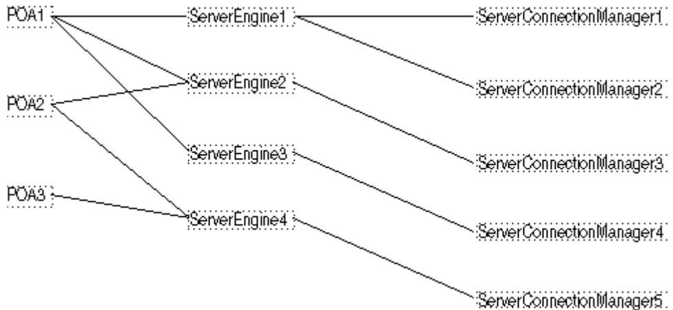
The simplest case is where POAs have their own unique single server engine. Here, requests for different POAs arrive on different ports. A POA can also have multiple server engines. In this scenario, a single POA supports requests coming from multiple input ports.
